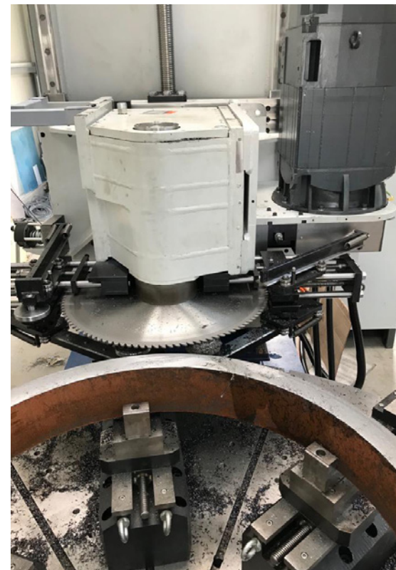
The prototype at Klaaßen Maschinenbau with that time exposed circular saw blade (Picture: Dango & Dienenthal)
