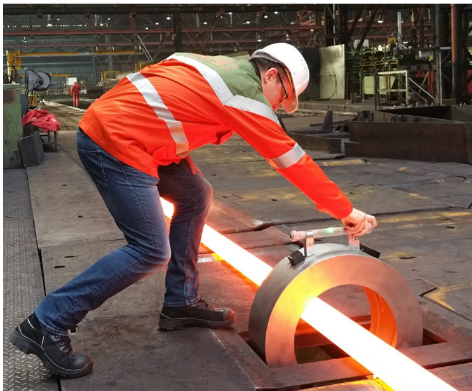
Profile gauge CALIPRI RC220 in the field at Mannstaedt GmbH (Picture: Nextsense)
