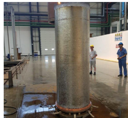
First remelted ingot at the new Ti-VAR plant at Chongqing Kingsley Titanium (Picture: INTECO)
