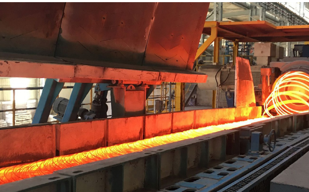
The laying head is equipped with oil-film bearings (Picture: Danieli)
