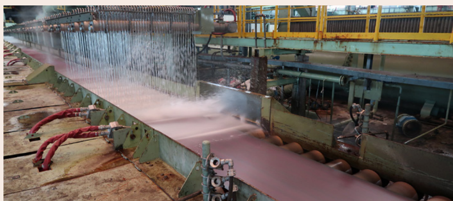
View of the reinforced laminar cooling and cross spray systems (Picture: SMS group)
