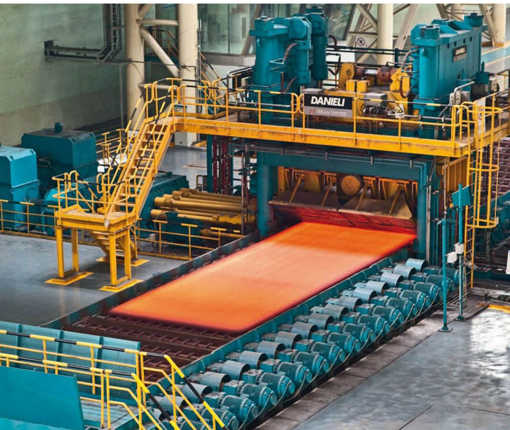
Plate being rolled in a reversing mill (Picture: Danieli)
