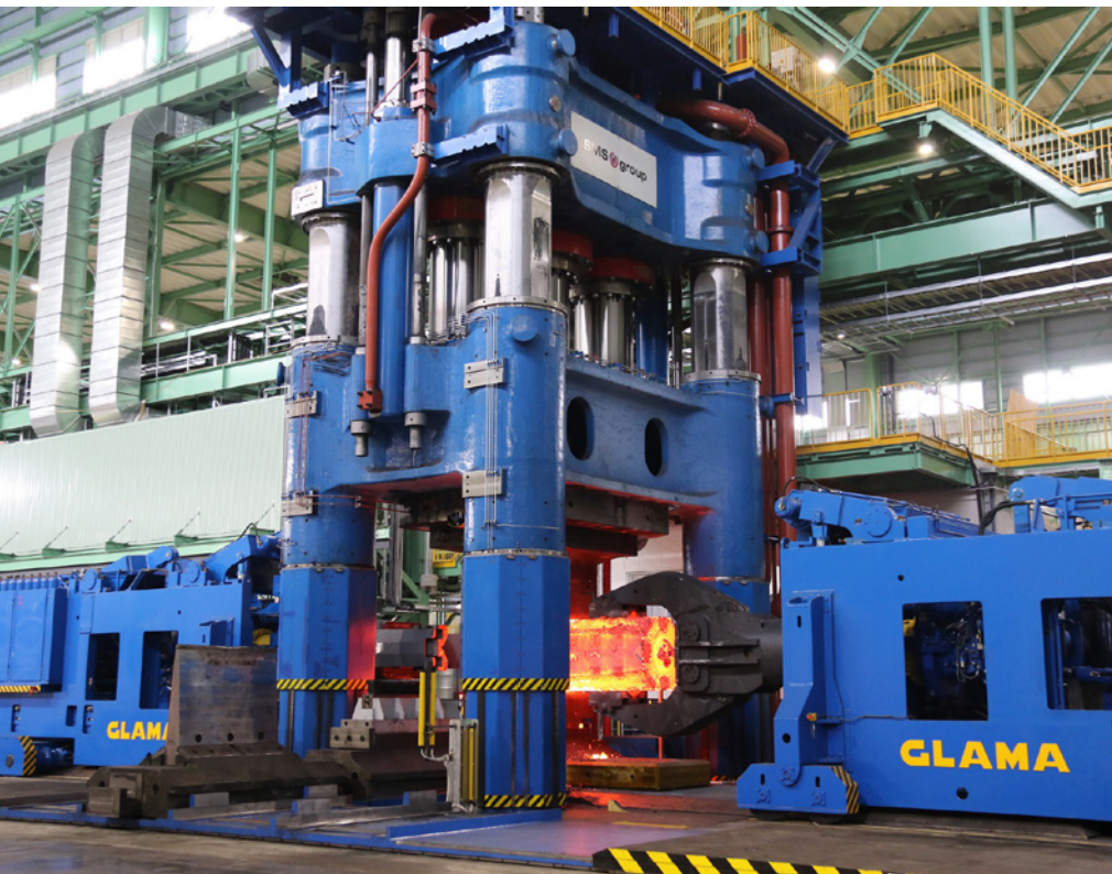
The 90/108 MN open-die forging press in operation at Hitachi Metal's Yasugi Works (Picture: SMS group)
