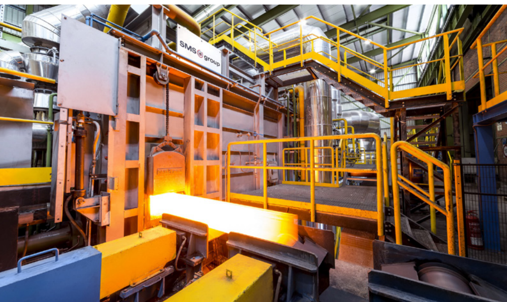
After the upgrade, the walking beam furnace at Basauri will have a capacity of 130 t/h (Picture: SMS group)
