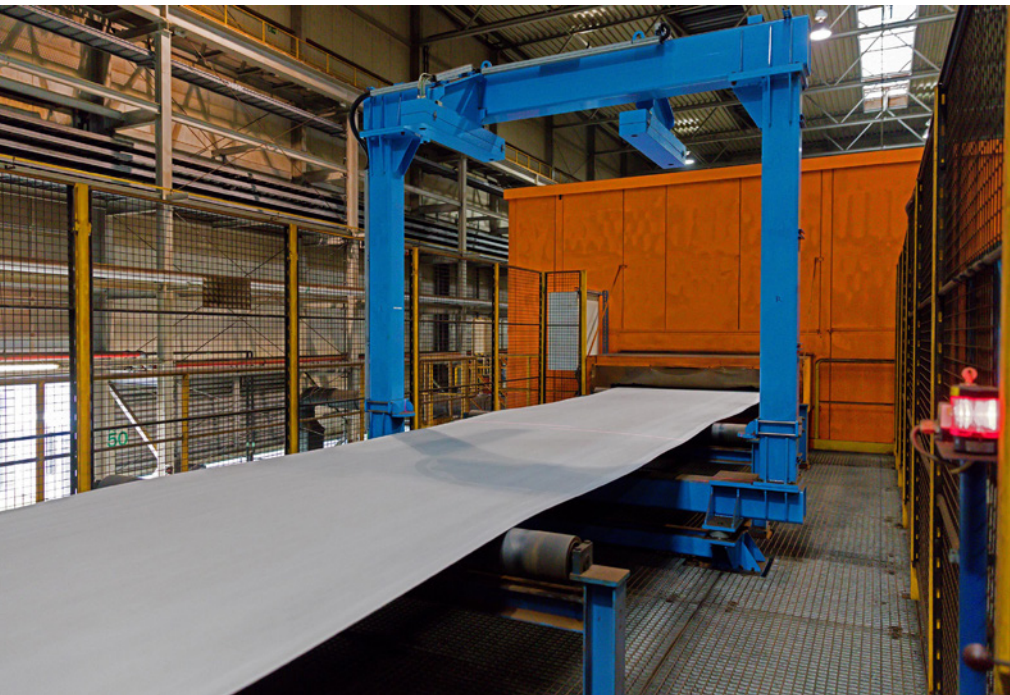
Crossbow measurement system at a continuous pickling line entry installed between the bridge roll and the process section (Picture: nokra)
