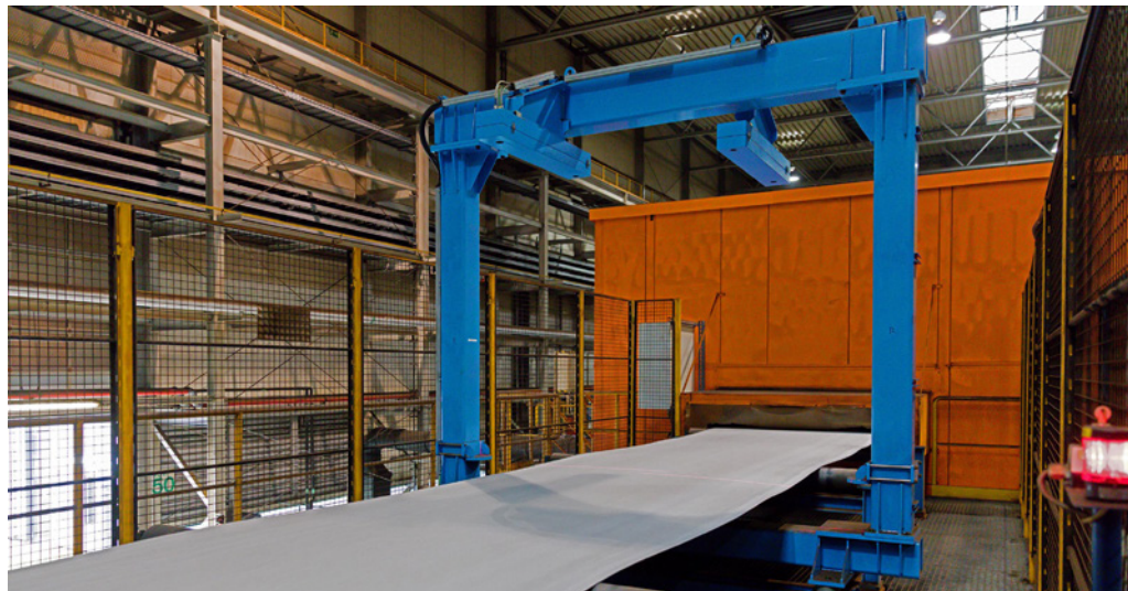
The exit gauge documents the crossbow of the pickled strip (Picture: Salzgitter Flachstahl)
