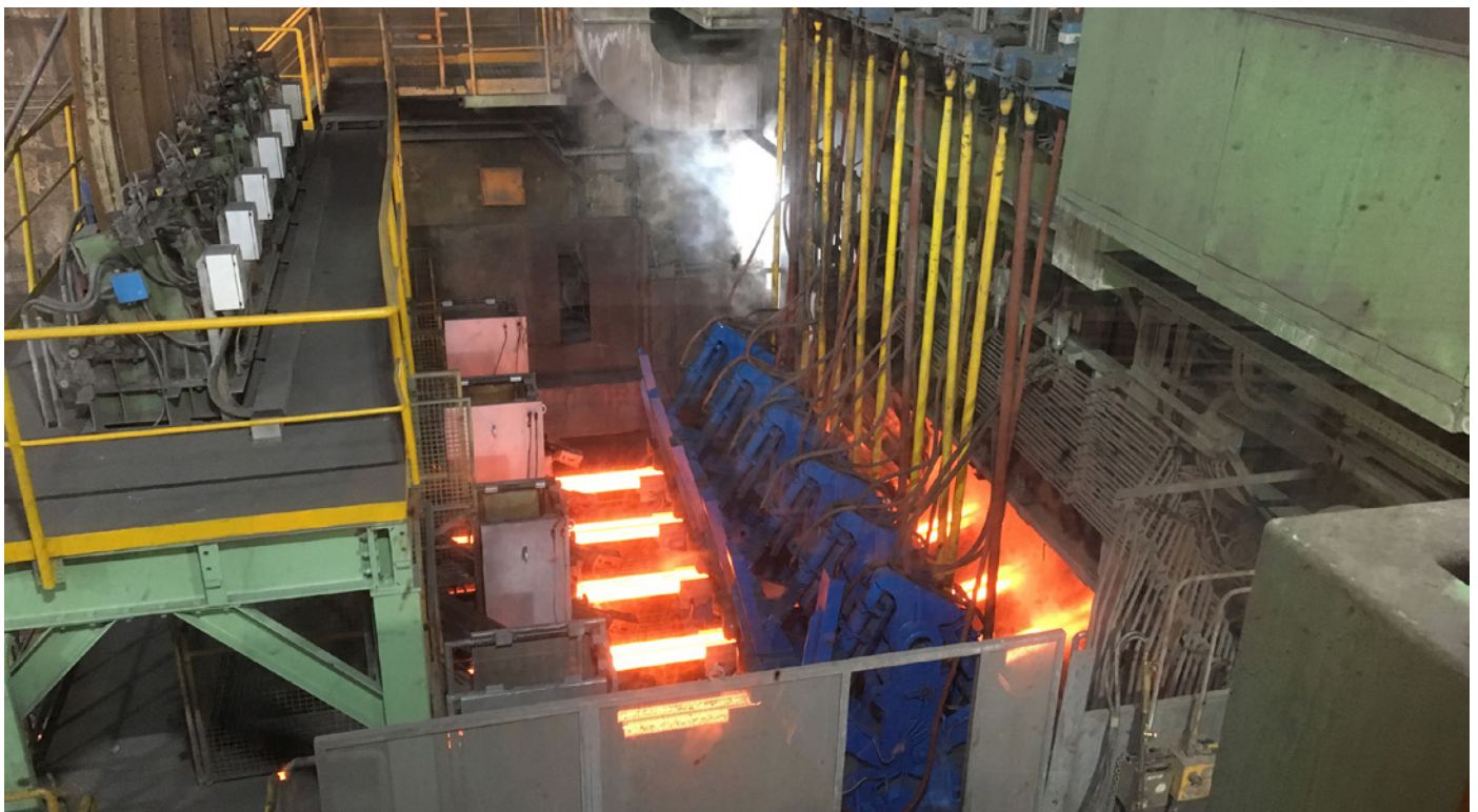
Continuous billet caster modernized by Primetals Technologies in the Lonato del Garda, Italy works of Feralpi Siderurgica (Picture: Primetals Technologies)
