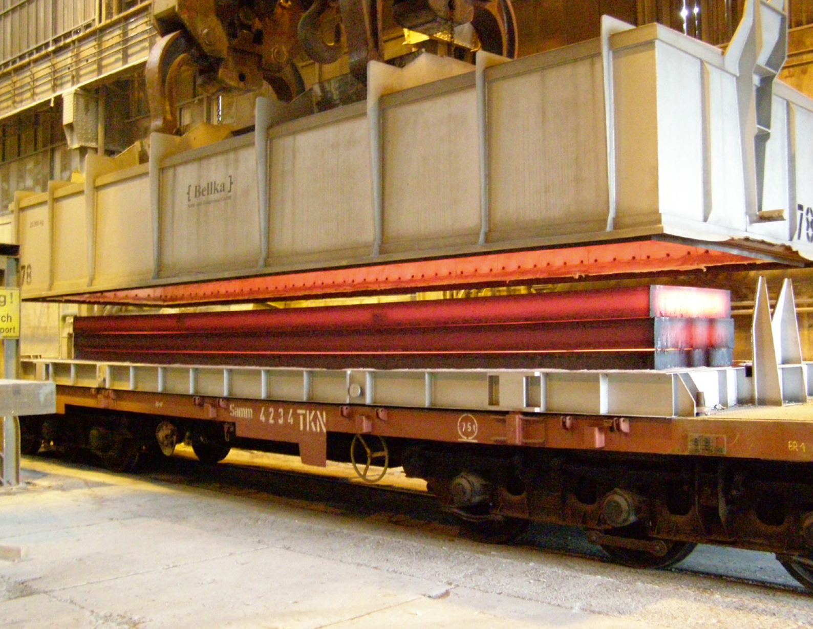
Figure 1. Hot transfer car with slabs (Picture: SMS group)
