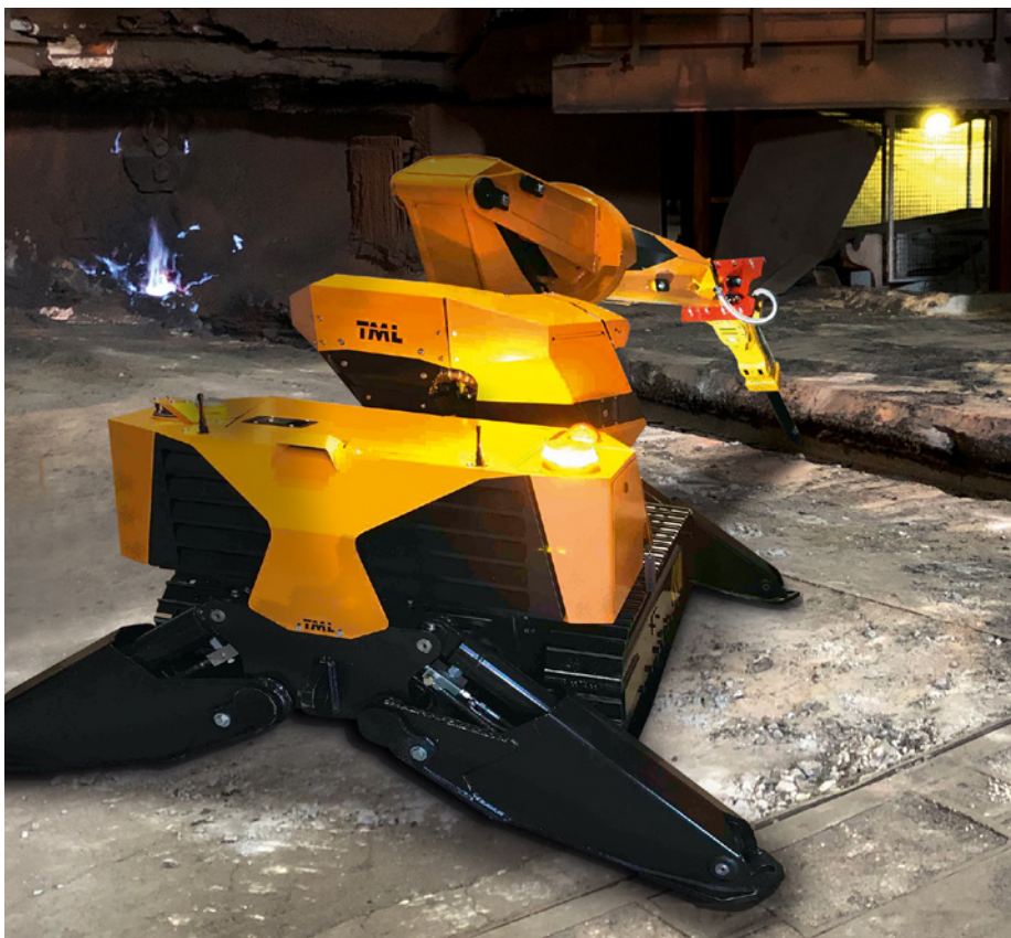
De-bricking of a blast furnace runner with Unidachs 100 (Picture: TML Technik)
