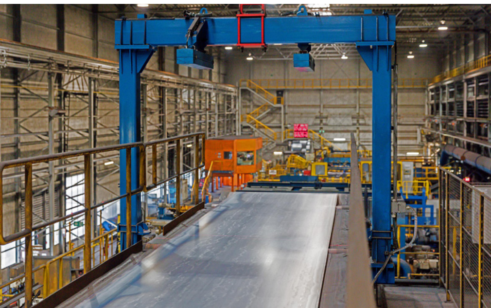
The entry gauge is arranged between the bridle rolls and the entry of the pickling section (Picture: Salzgitter Flachstahl)
