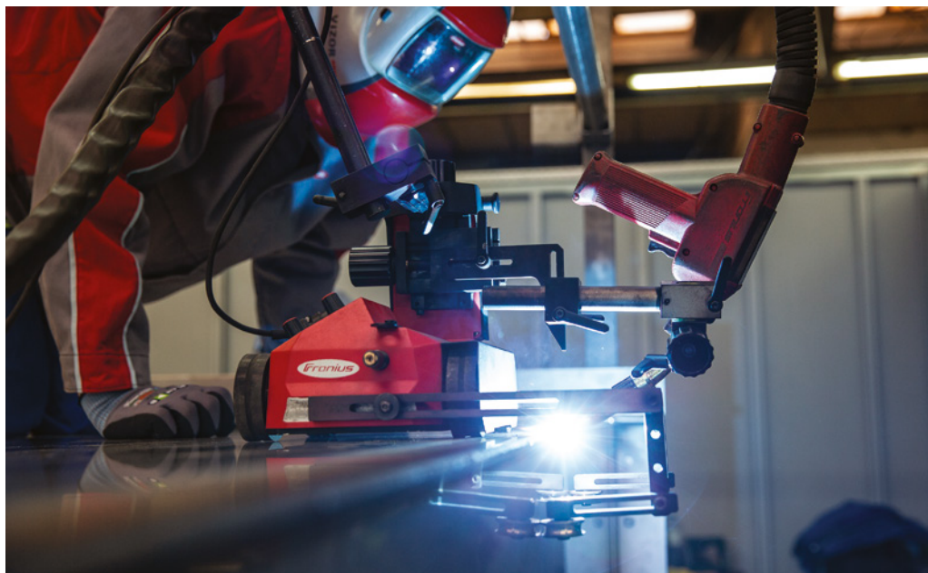
The ArcRover 22 welding carriage with guide rails welds a longitudinal seam (Picture: Fronius)
