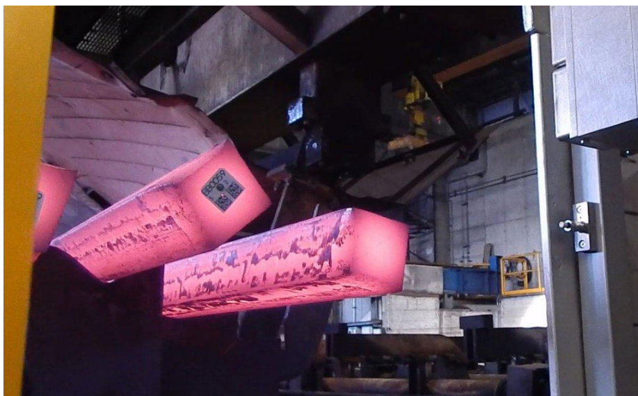
Billet just tagged on the cooling bed with PolyTAG (Picture: Polytec)
