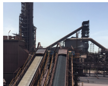
Conveyor belt for pellet cooling and transport (Picture: Aumund)
