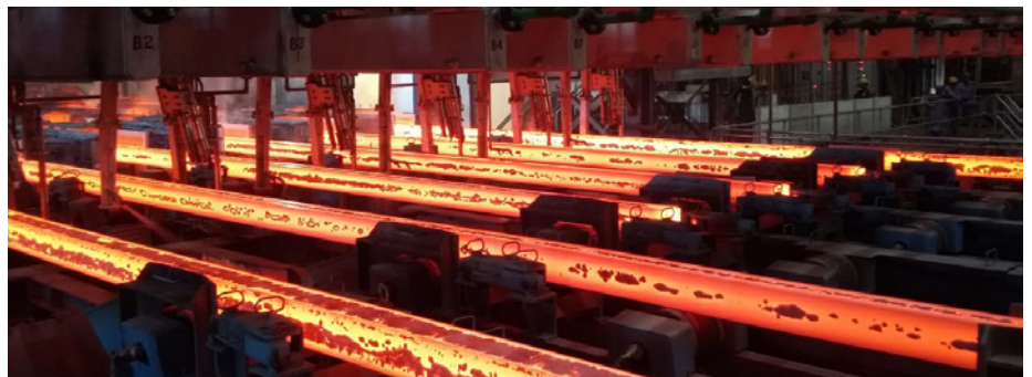
New high-speed billet caster operating at Jindal Shadeed Iron & Steel shortly after start-up (Picture: SMS group)
