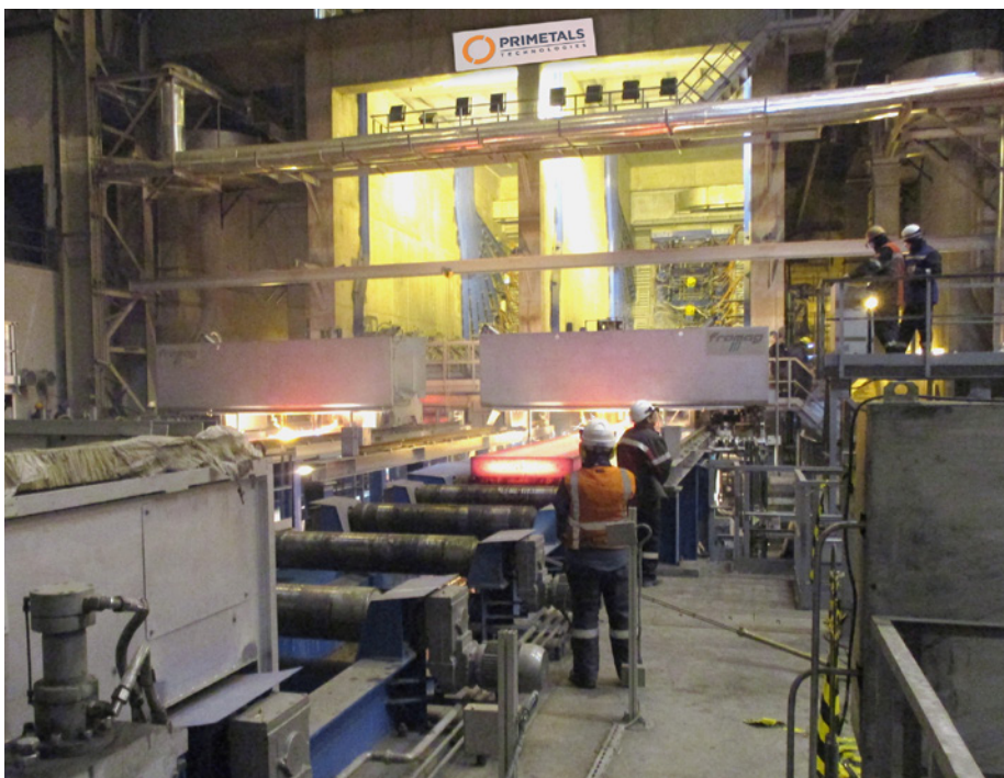
The two-strand caster CC4 is designed to produce 2.5 million t of slabs per year (Picture: Primetals Technologies)
