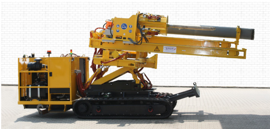
The universal machine KBSE performs all operations necessary for the tapping and maintaining of the converter: core-hole drilling, repair and mudding (Picture: Maschinentechnik Roth)
