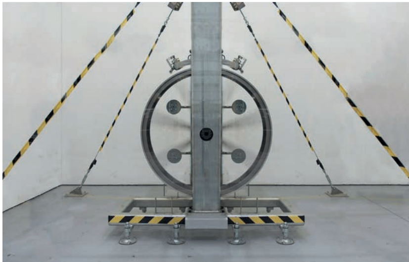
A testing facility in the form of a spinning wheel that can reach linear speeds of up to 500 km per hour (Picture: Zeleros)
