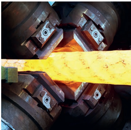
Figure 2. Close-up view of the radial forging process (Picture: SMS group)
