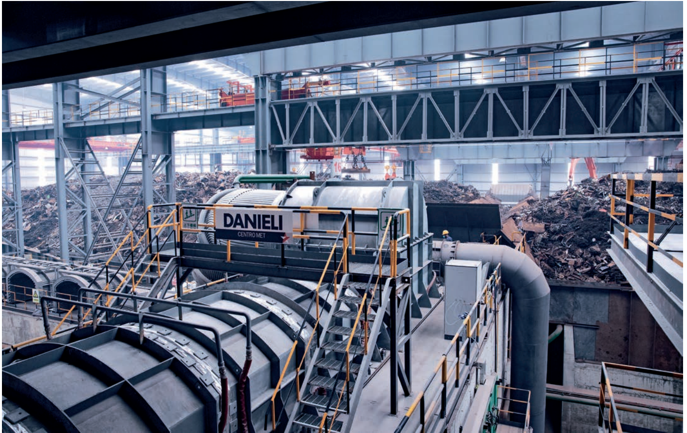
Zerobucket® ECS continuous scrap charge is characterized by low energy consumption, lowest noise and pollution emissions
