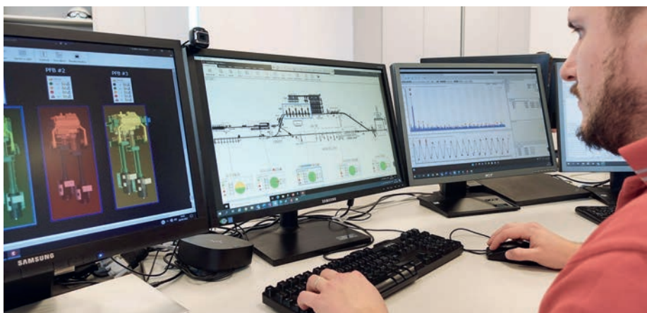
HMI of the condition monitoring system (Photo: Danieli)
