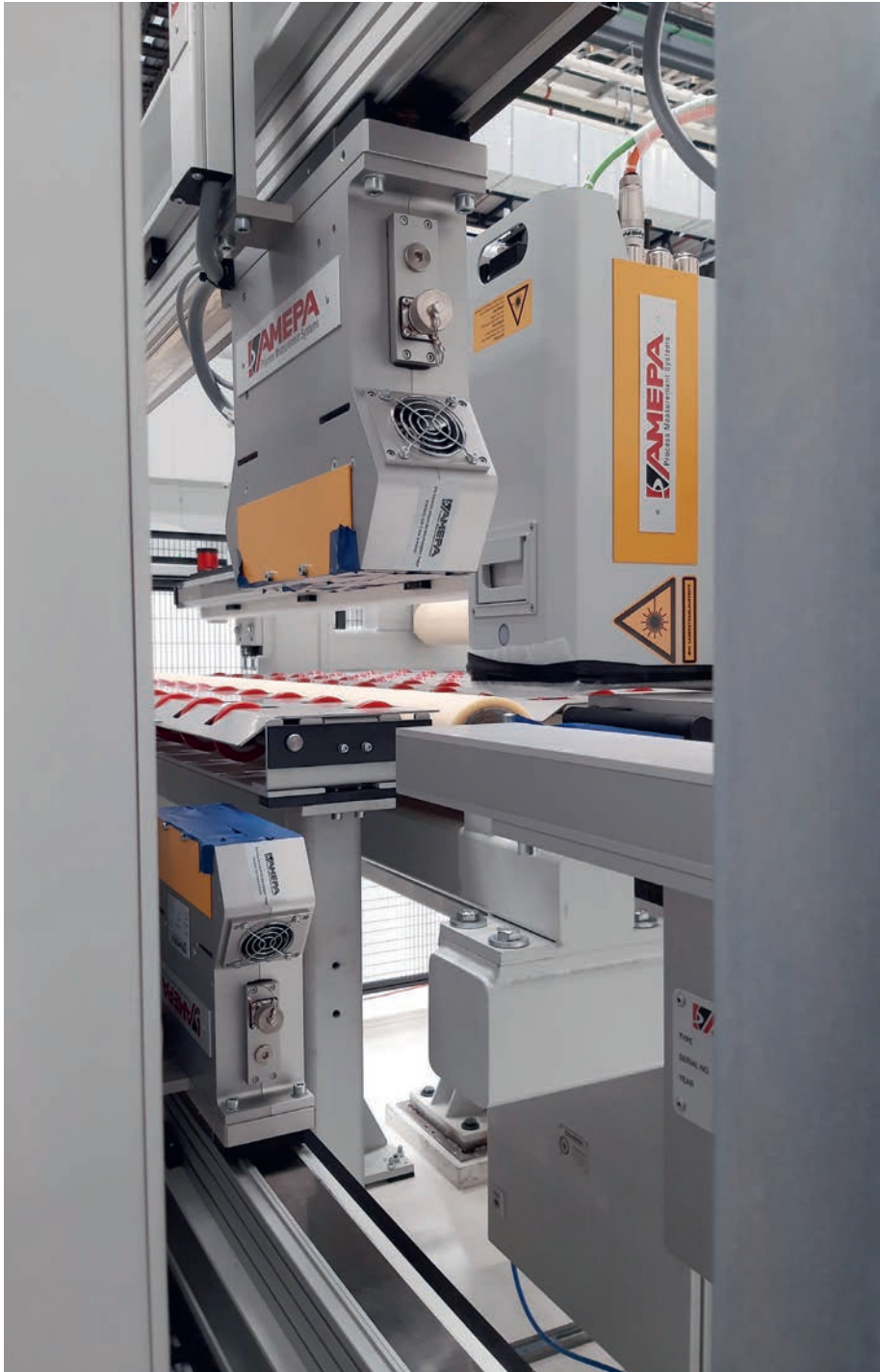
Moving across the entire width of the strip, the sensors measure the oil film (left) and the surface roughness (right) (Picture: Amepa GmbH)
