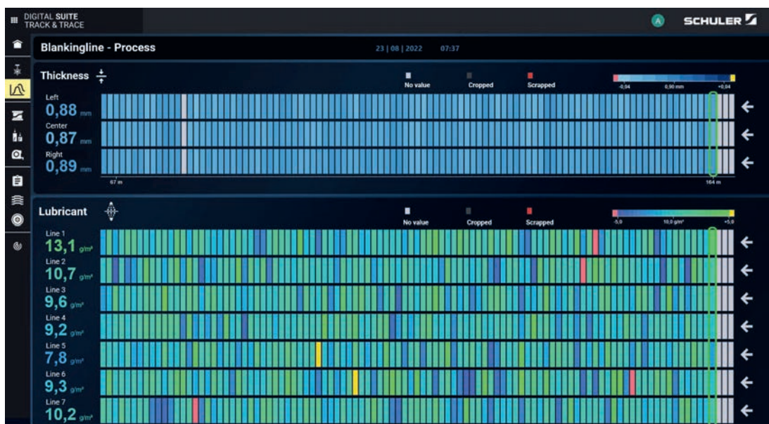
The measured values are graphically displayed in a clearly structured form by meter of strip (Picture: Schuler Pressen GmbH)
