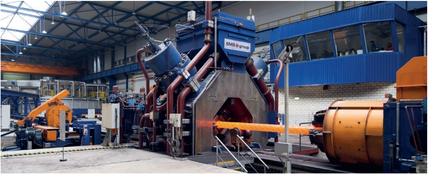
Figure 1. Hydraulic radial forging machine in operation (Picture: SMS group)
