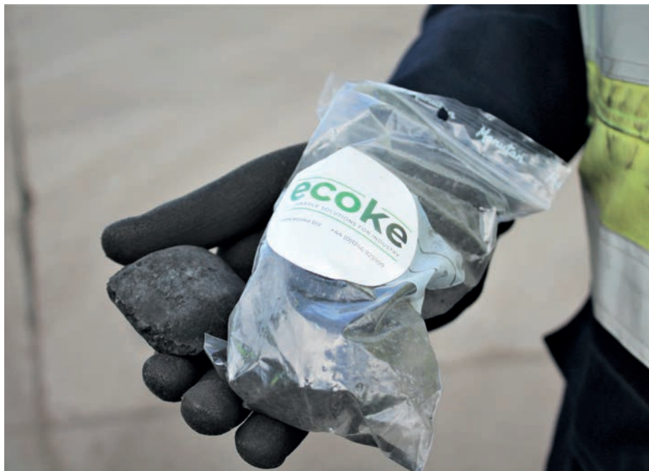
The briquettes are delivered to site in similar packaging to the anthracite and ecoke is charged into the EAF in the same manner via the scrap basket (Picture: Liberty Steel)
