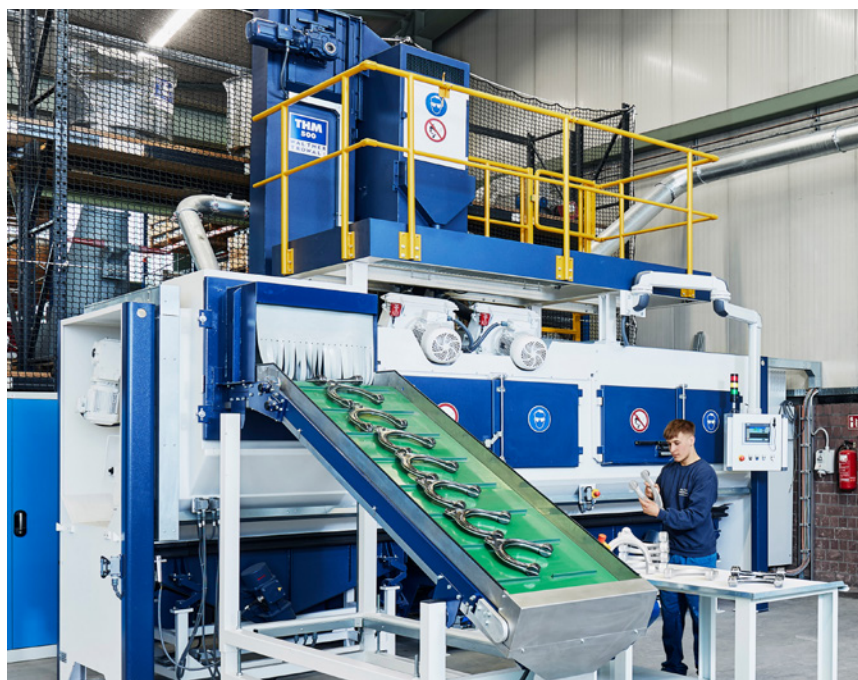
A THM 500 troughed belt continuous flow shot blast machine in the Trowal test and training center in Haan/Germany.
