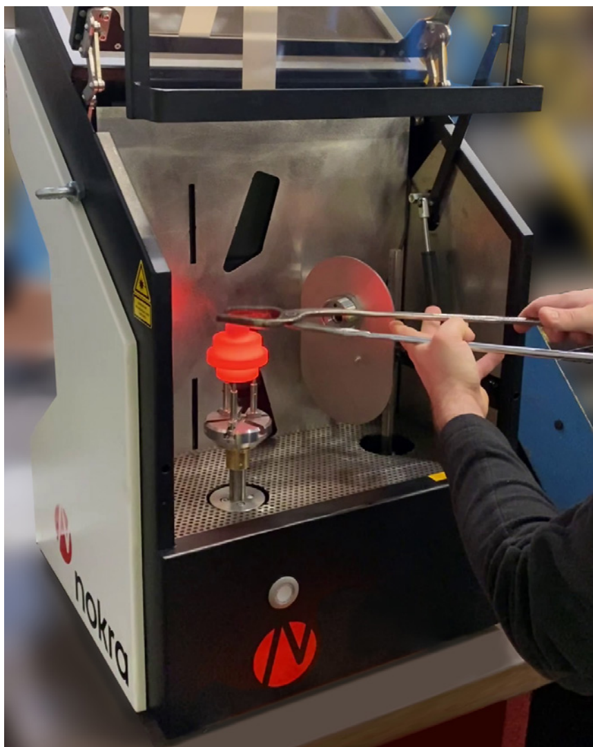
The hot forged parts are picked up by a conveyor belt as they leave the forging press and directly placed into the measuring cell.
