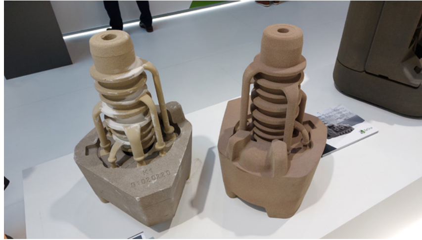
Comparison between a conventional, multi-part sand core (left) and a core produced in one piece using the 3D process (right).
