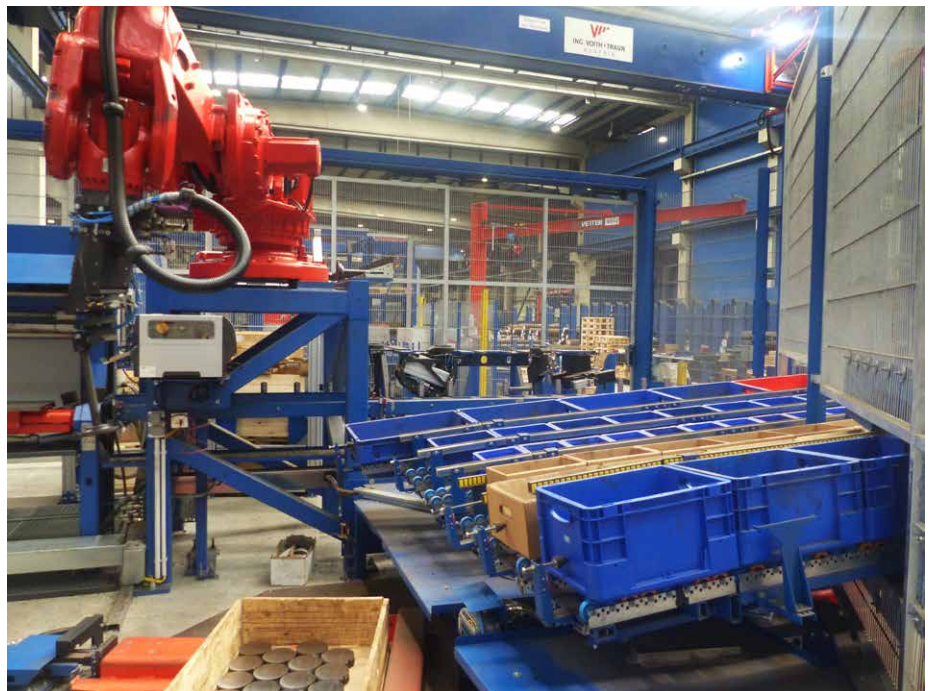
The robot at the saw loads the pallets automatically; the employees are then only responsible for securing the load (Picture: Kasto)
