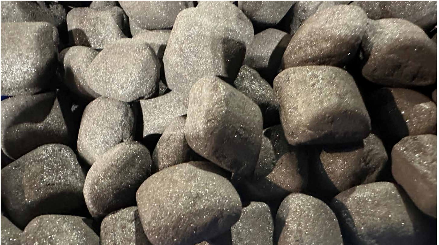
Using cold-bonded pellets has the potential to significantly reduce CO 2 emissions in ironmaking (Picture: Binding Solutions Limited)
