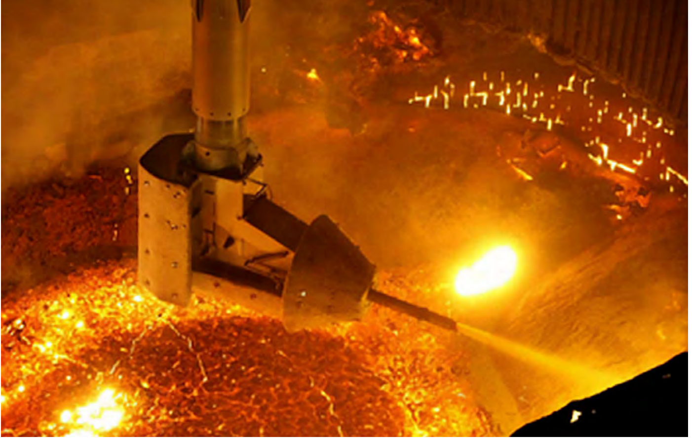
Figure 2. MINSKAN™ gunning head in operation (Picture: Minteq)
