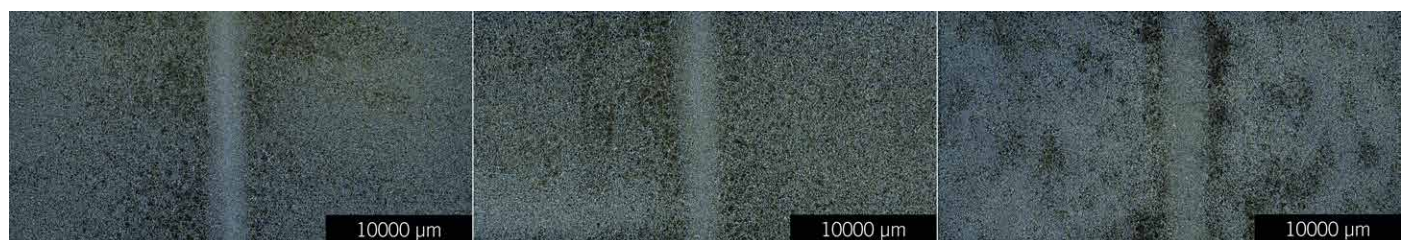
Figure 6. Macroscopic view of metallographic specimens of C35CrB; left: at surface, middle: 30 mm from surface, and right: 80 mm from surface (1/2 L of billet, core)
