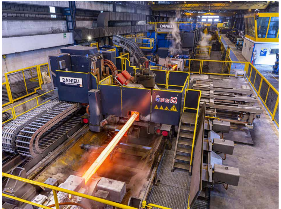
Figure 1. Horizontal billet welder in operation (Picture: Danieli)
