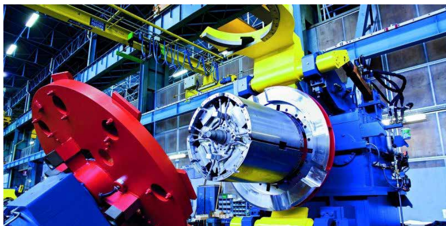
Spooler technology for the production of compact rebar coils (Photo: Danieli)
