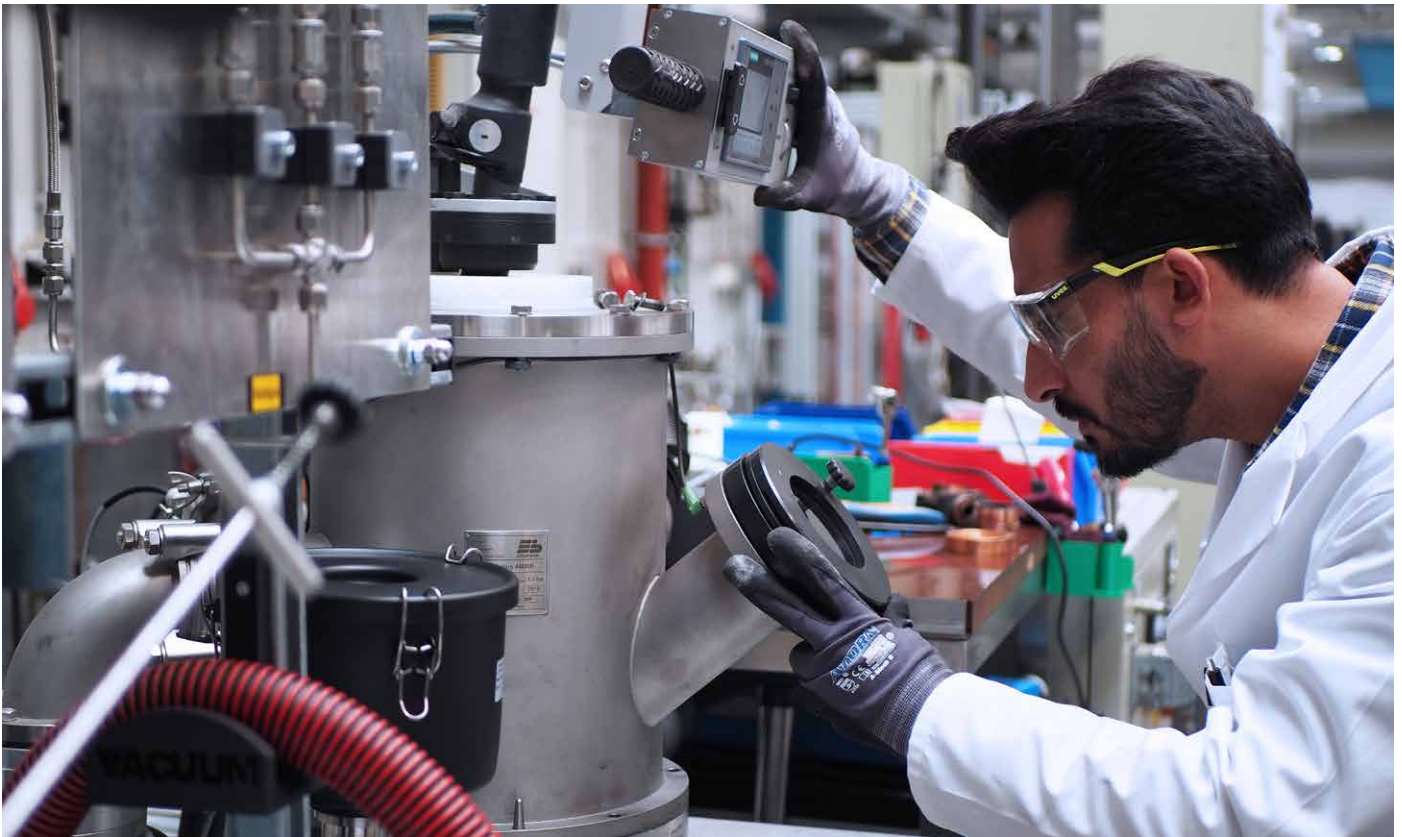
Ubaid Manzoor using an electric arc furnace to reduce low-grade nickel ores with hydrogen plasma
