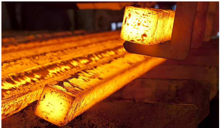
The new 7-strand continuous caster at IDC's steel works in Aliağa, İzmir, Türkiye is designed to produce billets and small blooms in six distinct section sizes (Photo: SMS group)
