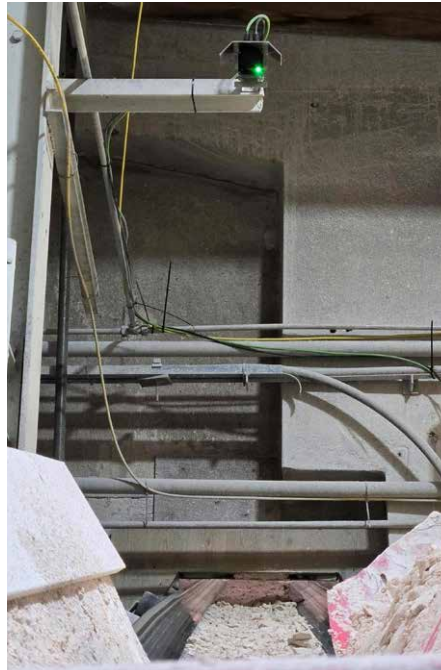
Mounted above the conveyor belt, the LiDAR sensor continuously scans the cross-sectional profile of the material (Picture: Sachtleben Technology)
