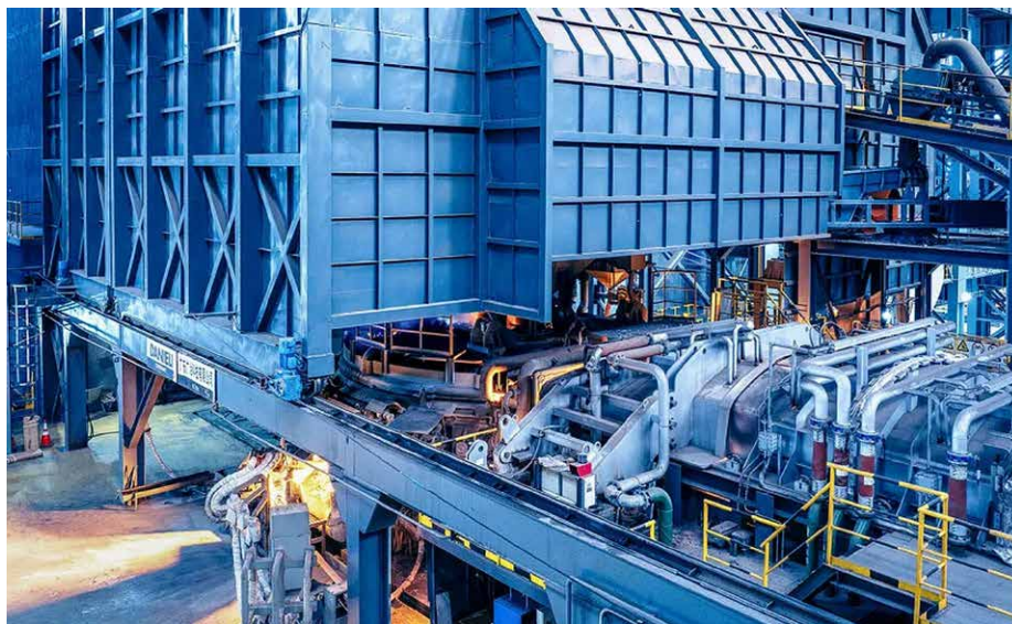
Electric arc furnace at Zhejiang Yuxin incorporating latest continuous scrap charging equipment (Picture: Danieli)
