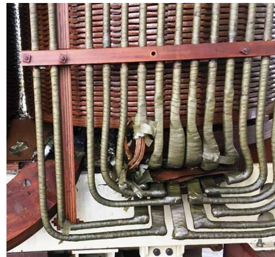
Figure 3. Destroyed HV regulating winding conductors at the bottom of the coil (Picture: BSE)
