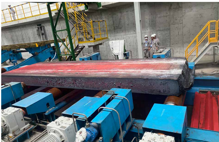
Wuyang Iron and Steel's new continuous caster is engineered to produce ultra-thick slabs up to 460 mm in thickness (Picture: Primetals Technologies)
