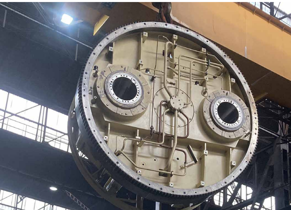
The service project involved removing the rotor, which has a diameter of four meters and weighs 55 tons (Picture: SMS group)
