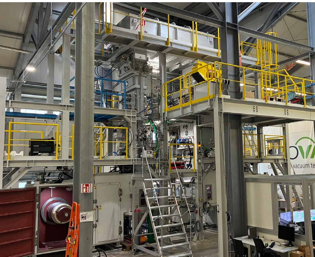
Pilot plant for the continuous coating of highly sensitive materials, such as martensitic steel strip (Picture: NEOVAC)
