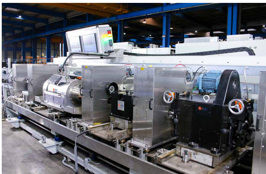
(From left to right:) Combined testing bench including rotating head RotoUTscan and rotating head RotoETscan (Picture: CMS)
