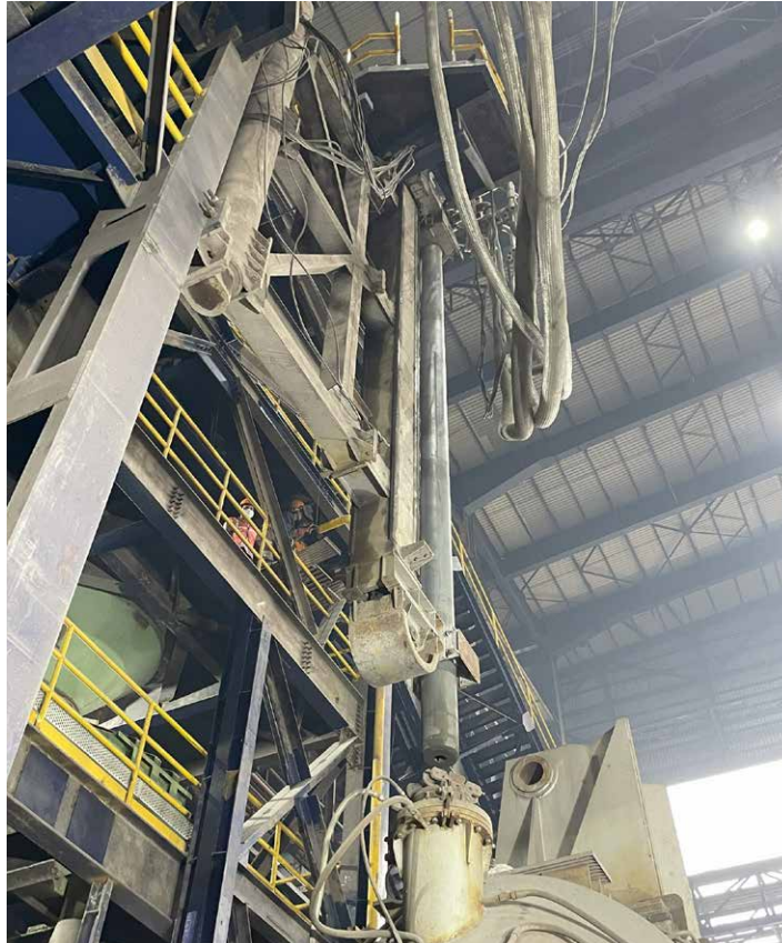
TOP-Lance of the RH plant at JSW Dolvi Works steelmaking shop 2 in Maharashtra, India (Picture: SMS group)
