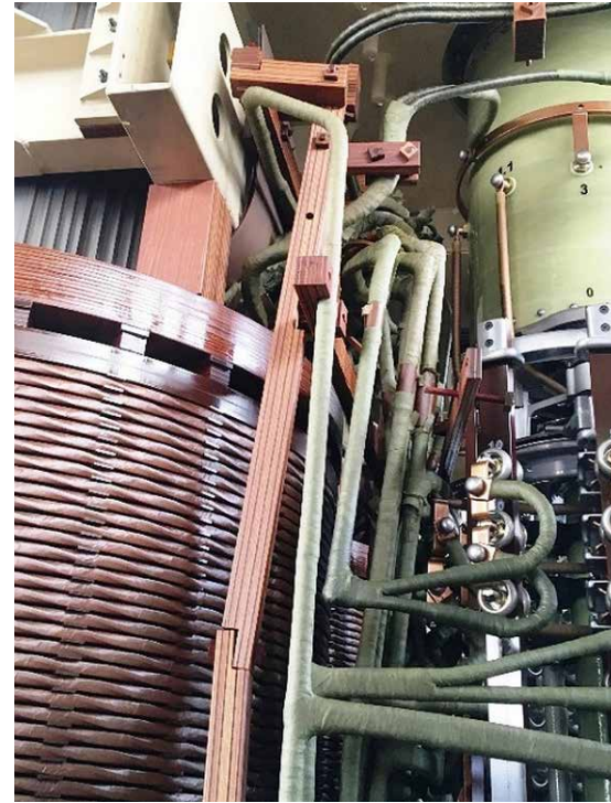
Figure 2. Destroyed HV regulating winding conductors at the top of the coil (Picture: BSE)
