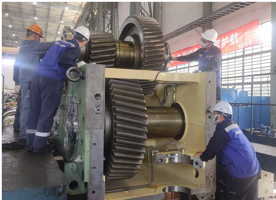
Overhaul of the gearboxes in the 2,050-mm hot strip mill at Baoshan Iron & Steel (Picture: SMS group)
