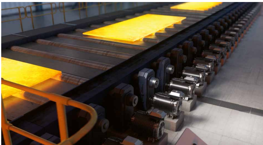
Aging DC motors on roller tables can be replaced with new AC motor-drive packages (Picture: ABB)
