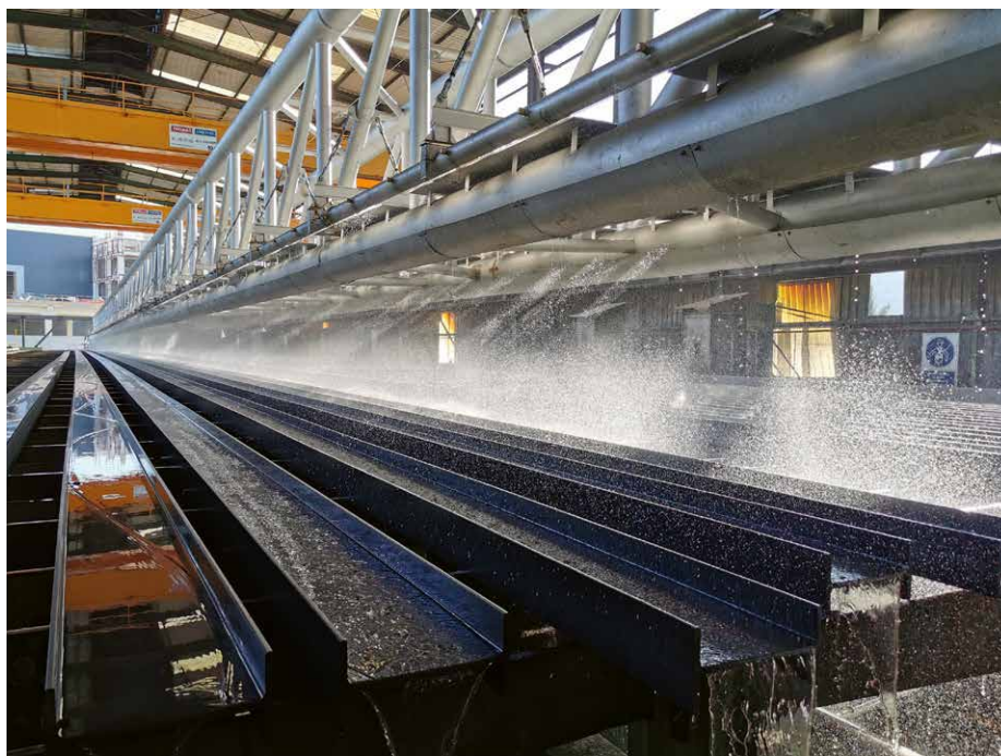
Celsa Barcelona's medium section mill produces a variety of long rolled products, including beams, angles and channels (Picture: SMS group)
