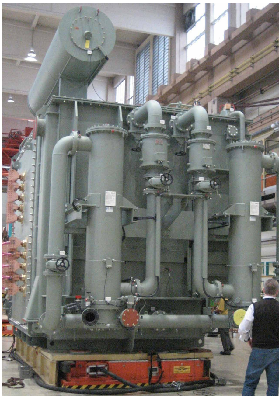
Figure 1. 150 MVA furnace transformer during the factory test (Picture: BSE)
