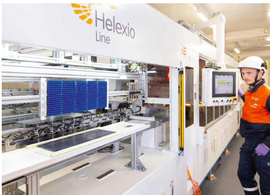
The top steel sheet of the sandwich panel is fitted with photovoltaic cells (Picture: ArcelorMittal)
