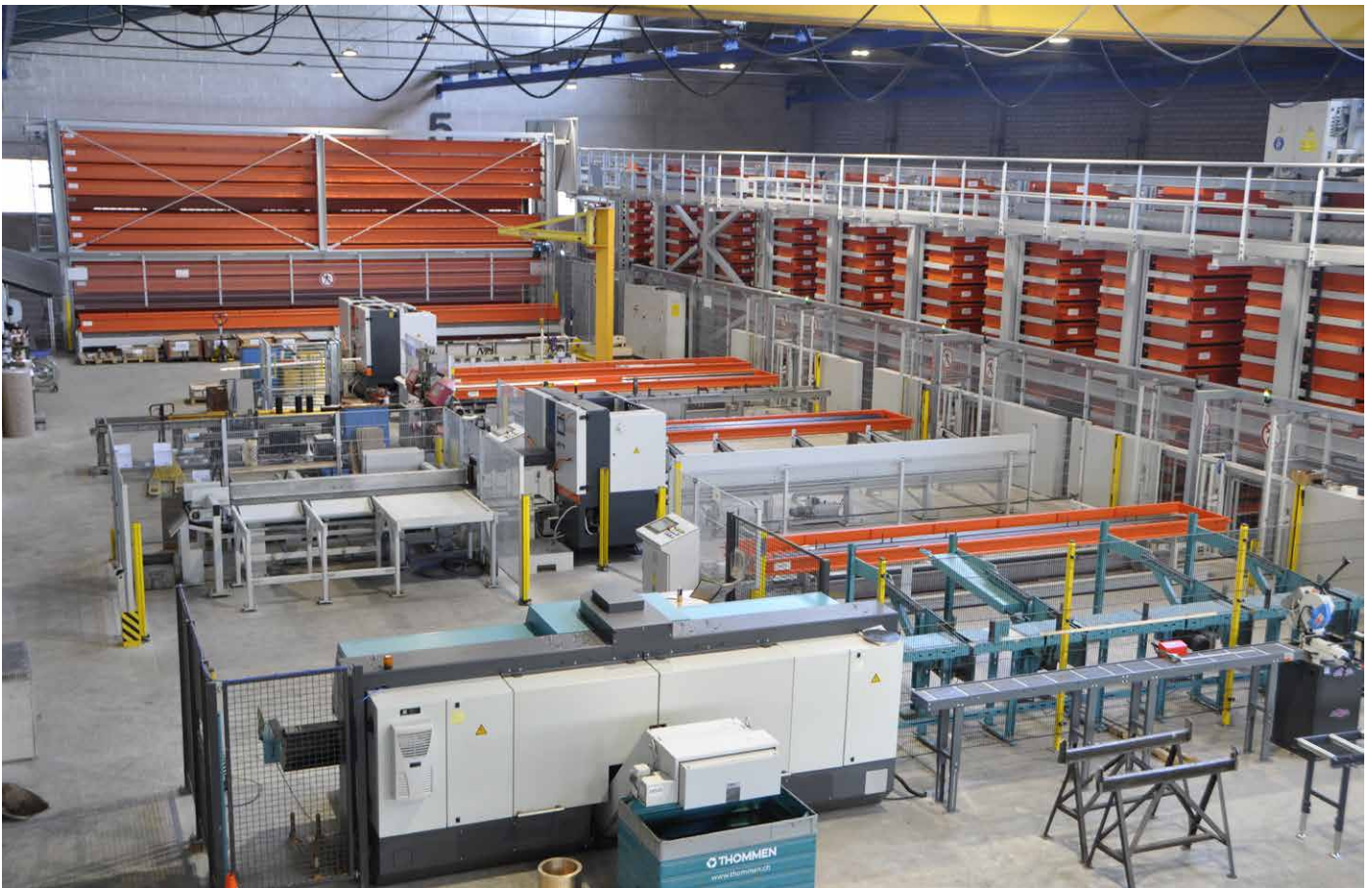
The combination of two automatic storage systems, high-performance output stations, and flexible sawing centres ensure short delivery times (Picture: Kasto Maschinenbau)
