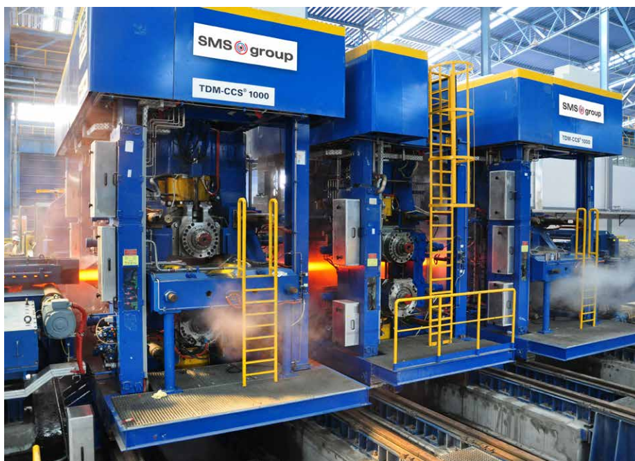
Compact cartridge stands in SULB's heavy section mill in Bahrain, supplied as part of the greenfield minimill project in collaboration with Yamato Kogyo (Photo: SMS group)
