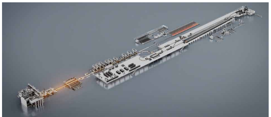
Layout of the new long-product mill ordered by UMB Steel (Photo: SMS group)
