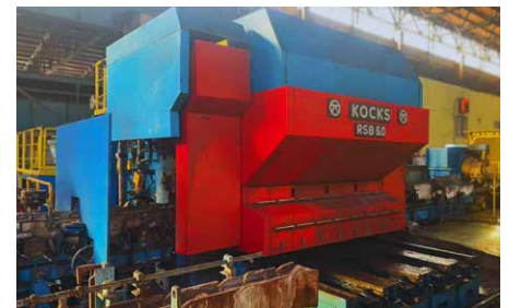
The reducing & sizing block has been successfully integrated into Fushun Special Steel's regular SBQ production (Photo: Kocks)
