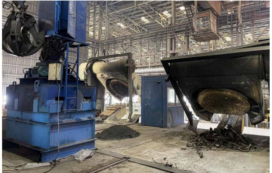
Setting at Al Qaryn Steel: IFM9 induction furnace (charged) with the Eco Top hood, with a charging crane beside it (Picture: ABP)
