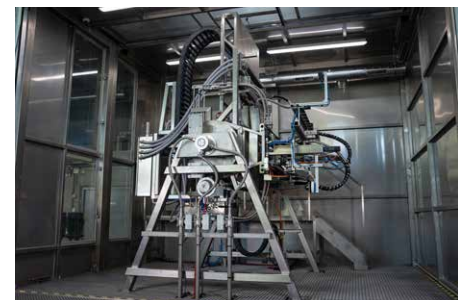
The flexible setup allows testing of any type of industrial cooling system (Picture: Primetals Technologies)
