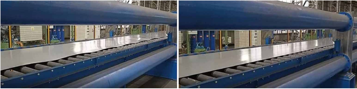
Stretching straightening technology significantly reduces the risk of unpredictable deformations after cutting (Picture: SSC Europe)
