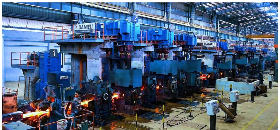
Jai Raj Ispat produces finished thermomechanically treated bars in an energy-efficient sequence (Photo: Danieli)
