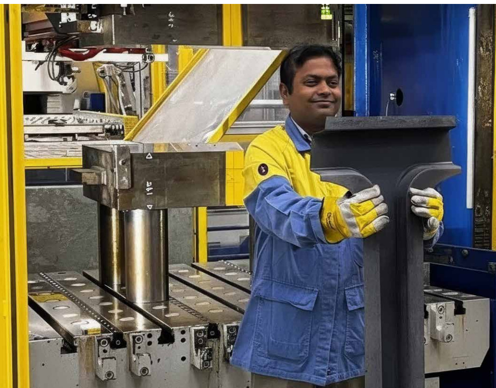
Dr Radhakanta Rana holding a hot press formed automotive steel component (Picture: Tata Steel Nederland)
