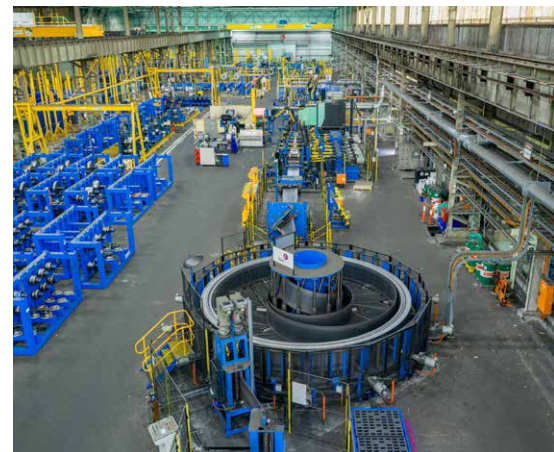
In addition to reducing manual handling, the automated process ensures repeatability, clean and consistent bundle formation, and lower noise levels (Picture: Fives)
