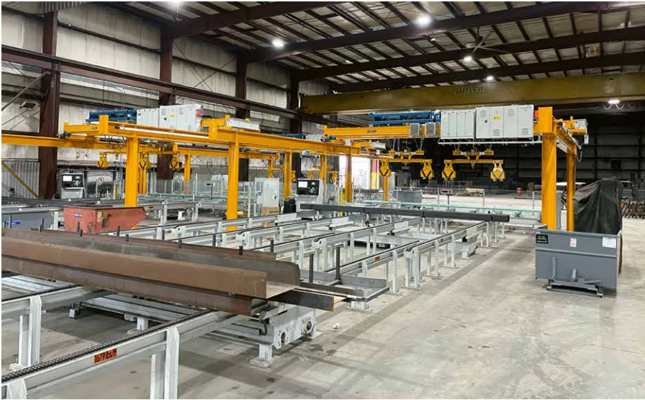
Thanks to intelligent circulation stations, infeed and outfeed speeds have significantly increased (Picture: Kasto Maschinenbau)
