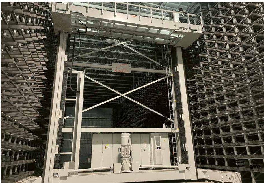
The honeycomb automatic storage and retrieval system maximises storage capacity and optimises use of the available footprint (Picture: Kasto Maschinenbau)
