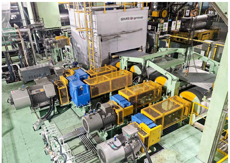
Modernized hot-dip galvanizing line after phase one, with new bridle rolls and a strip dryer (Picture: SMS group)
