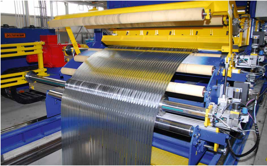
The slitting shears produce accurate, low-burr cuts, even when numerous narrow slits need to be made (Picture: GEORG)
