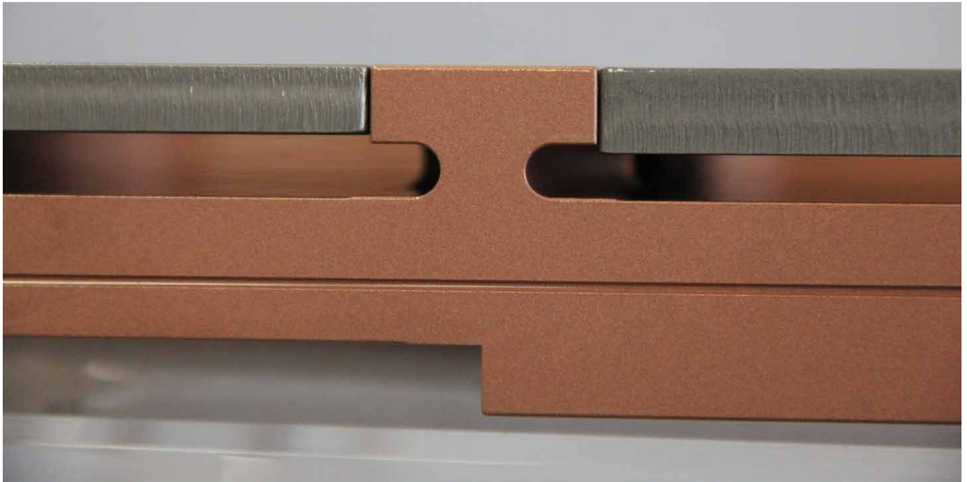
Figure 6. The filler pieces create variable water gaps that allow precise control of local flow and heat dissipation conditions (Picture: cunova GmbH)
