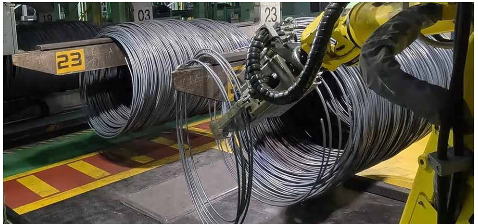
TrimRob autonomous coil trimming and sampling robot (Picture: Primetals Technologies)
