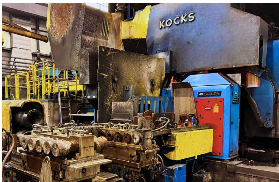
Advanced laser-based measuring system integrated in Steeltec's rolling mill (Photo: Kocks / LAP)
