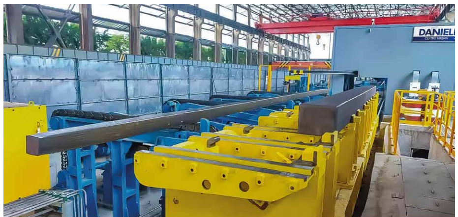
Billet grinding machine in operation (Photo: Danieli)
