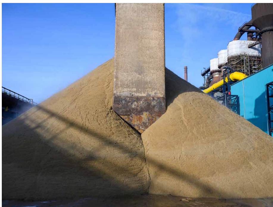
Granulated slag is a recycled material that is commonly used in cement production (Picture: FEhS-Institut/Michael Wieschke)
