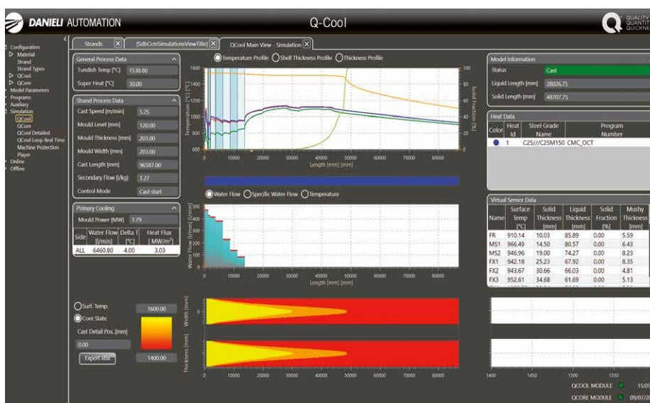
The Q-Cool solidification model monitors and dynamically controls the cooling parameters and product solidification (Picture: Danieli)
