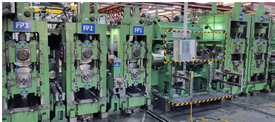
The forming and welding area of Tuflesa's ERW tube line first upgraded in 2024 (Photo: SMS group)
