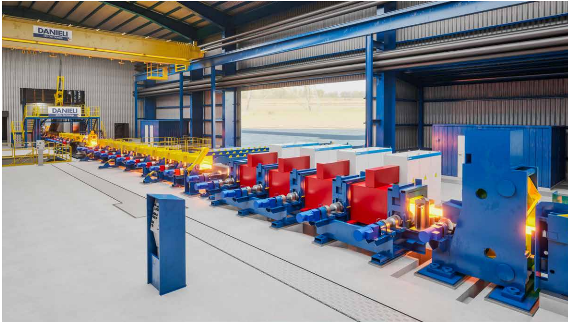
The Octocaster®, which is directly linked to the rolling mill, produces endless billets at speeds of up to 10 m/min (Picture: Danieli)
