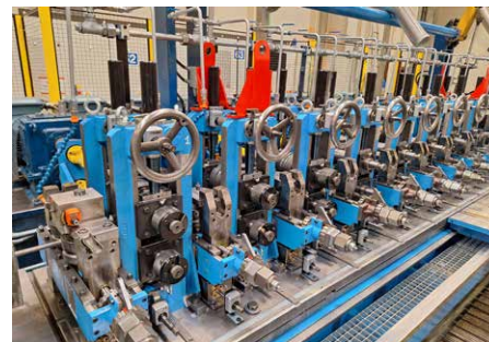
Aceros Arequipa will produce up to 40 mm tubes on its new OTO mill (Photo: Fives)
